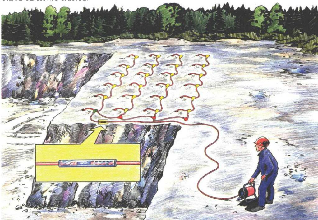
The *Exel™ Lead in Line* tube is connected to the *Exel™* rounds by means of an approx. 4 cm long outer tube that is cut from the transparent tube delivered with the *Exel™ Lead in Line* bobbin.
