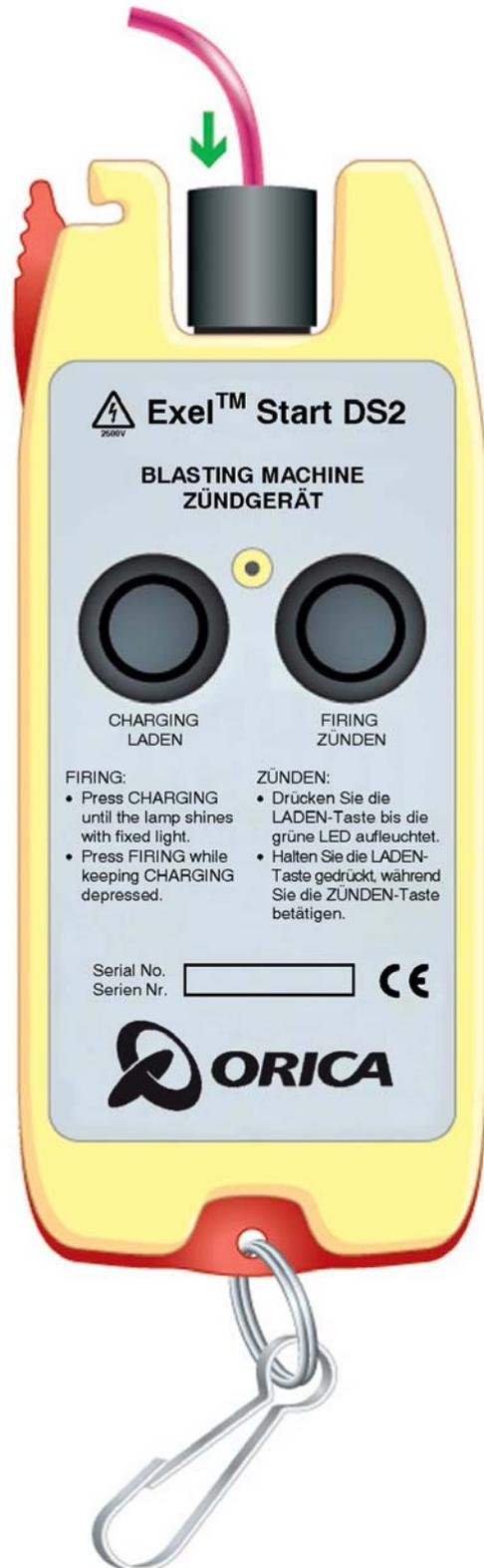
The *Exel™ Start DS2* is a further refined electronic blasting machine for the safe initiation of *Exel™* detonators. It consists of an energy source (battery), a voltage converter, a capacitor for energy accumulation, an electrode and pushbuttons to effect initiation. The electrical energy is converted to a powerful spark, which the electrode emits into the inside of the *Exel™ Lead in Line* tube to initiate the shock-wave reaction.
